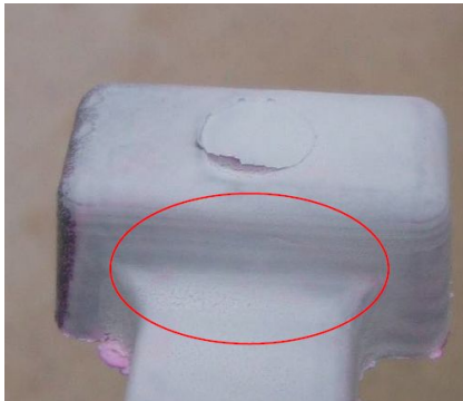
Fig. 7: Penetrant crack testing on an test casting out of the alloy AlSi14Cu4Fe1,8Cr0,3Mn0,1
