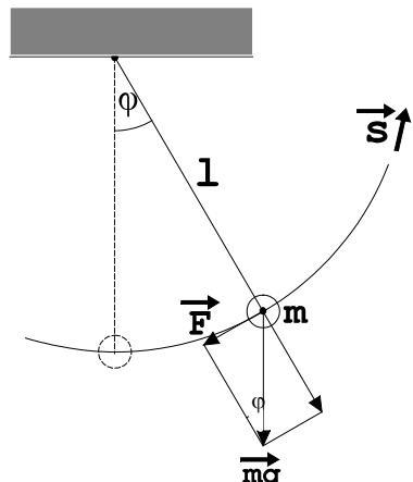
Using  $s = l \varphi$ , Newton's second law gives the equation of motion (acceleration  $a$  has the opposite direction to the deflection  $s$ ):
