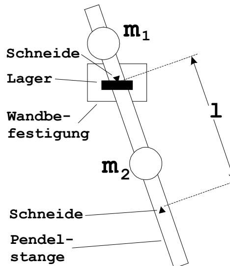
The reverse pendulum consists of a metal rod with two movable metal discs and two opposing edges as suspension devices. The distance between the two edges is engraved on the back of the pendulum. One metal disc with a mass of  $m_2 = 1400\text{g}$  can be moved between the two edges, and the other disc with a mass of  $m_1 = 1000\text{g}$  can be moved outside of one edge.
