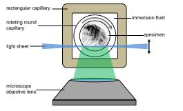
A light sheet is created perpendicular to the observation path either by a cylindrical lens [1] or by scanning of a laser beam. At SPIM only the plane under investigation is exposed to light, and successive measurements can be performed at low exposure of the whole sample when either the light sheet or the specimen is shifted in axial direction.
