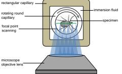
For illumination of the specimen a laser beam is focused by the microscope objective lens into the image plane and shifted by a scanning head to generate a 2-dimensional image. By moving the objective lens in vertical direction one can also generate a 3-dimensional dataset (optical sectioning).
