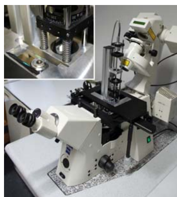
Figure 1. Illumination device for light sheet based fluorescence microscopy coupled to an inverse microscope (inlays: illumination of a spheroid within a micro-capillary).
