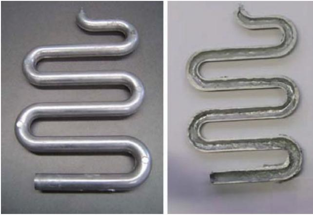
Figure 11 – Two casting geometries produced with gas injection.
