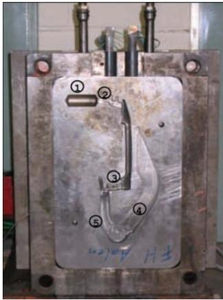
Figure 5 – Test die for high pressure die castings with gas injection; 1) Side Cavity; 2) Valve; 3) Gas Injector; 4) Gating 1; 5) Gating 2.
