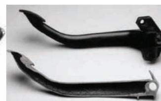
Figure 4 – Hollow structures in clutch pedal.
