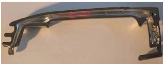
Figure 7 – Die casting produced by gas injection<sup>6,7</sup>.
