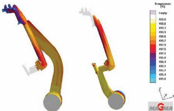
Figure 6 – Simulation of die fill indicating cold metal in the vicinity of the gas injector for Gating 1 (left) and optimized metal temperatures for Gating 2 (right).
