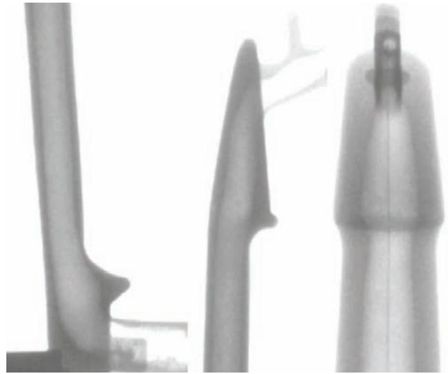
Figure 8 – X-ray of gas injected parts.
