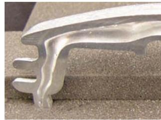
Figure 9 – Smooth surface of gas injected parts.
