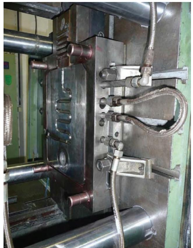
Figure 10 – Complete die set up in the die casting machine.
